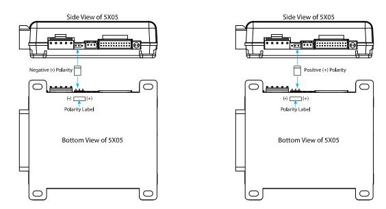
**Note 1**: The light flash polarity label can be found on the bottom of the 5X05 housing in the location shown in the above diagram.
