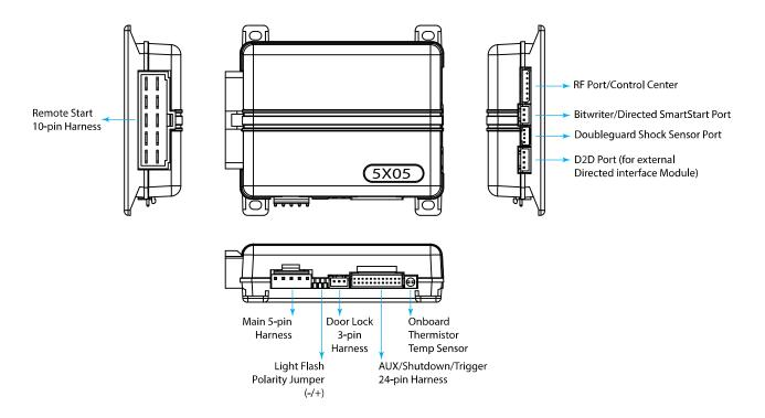
Note: (+) or (-) light flash jumper needs to be installed for the appropriate light flash polarity and is found taped to the outside on the main unit.
