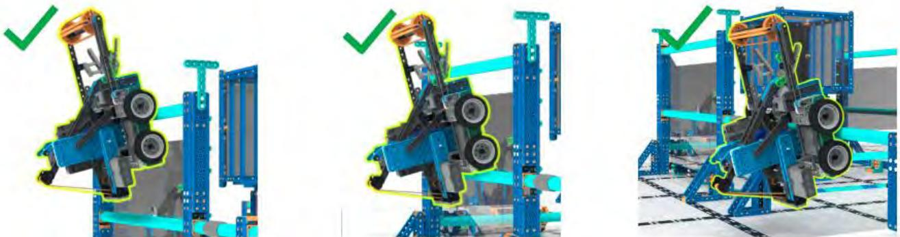
**Hanging Bar** - - One of the teal PVC pipes, 0.84" (21.3mm) in diameter, that run parallel to the Starting Corrals. The bottom edge of the highest set of Hanging Bars is 15.5" (393.7mm) from the Floor; the bottom edge of the lower set of Hanging Bars is 7.5" (190.5mm) from the Floor.
