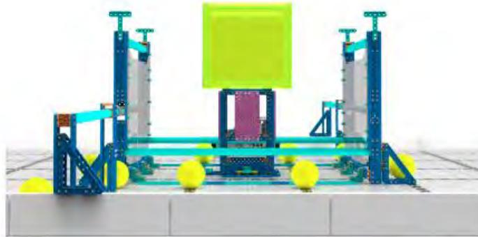
**Low Goal** - The area in the center of the Field surrounding the High Goal. On two sides, the Low Goal is bound by clear plastic sheets. On the other two sides, the Low Goal is bounded by the outer edge of the teal PVC pipes, and the VEX IQ parts attached to the Floor. The plastic sheets, PVC pipes, and VEX IQ parts are considered part of the Low Goal.
